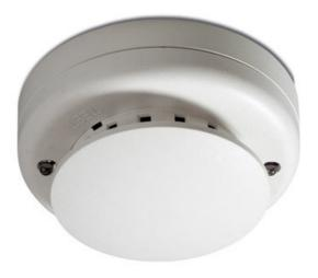
It samples the temperature in the protected zone with immunity to false alarms . It fitted with integrated isolator. It has three different colors LEDs for differents events: alarm condition (red) fault (yellow) and location (green)
