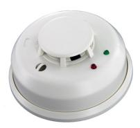
Multi criteria detector addressed with digital communication protocol . It can sample the temperature and to analys the conditions of air in the protected zone with immunity to false alarms . It fitted with integrated isolator. It has three different colors LEDs for differents events: alarm condition (red) , fault ( yellow) and location (green )
